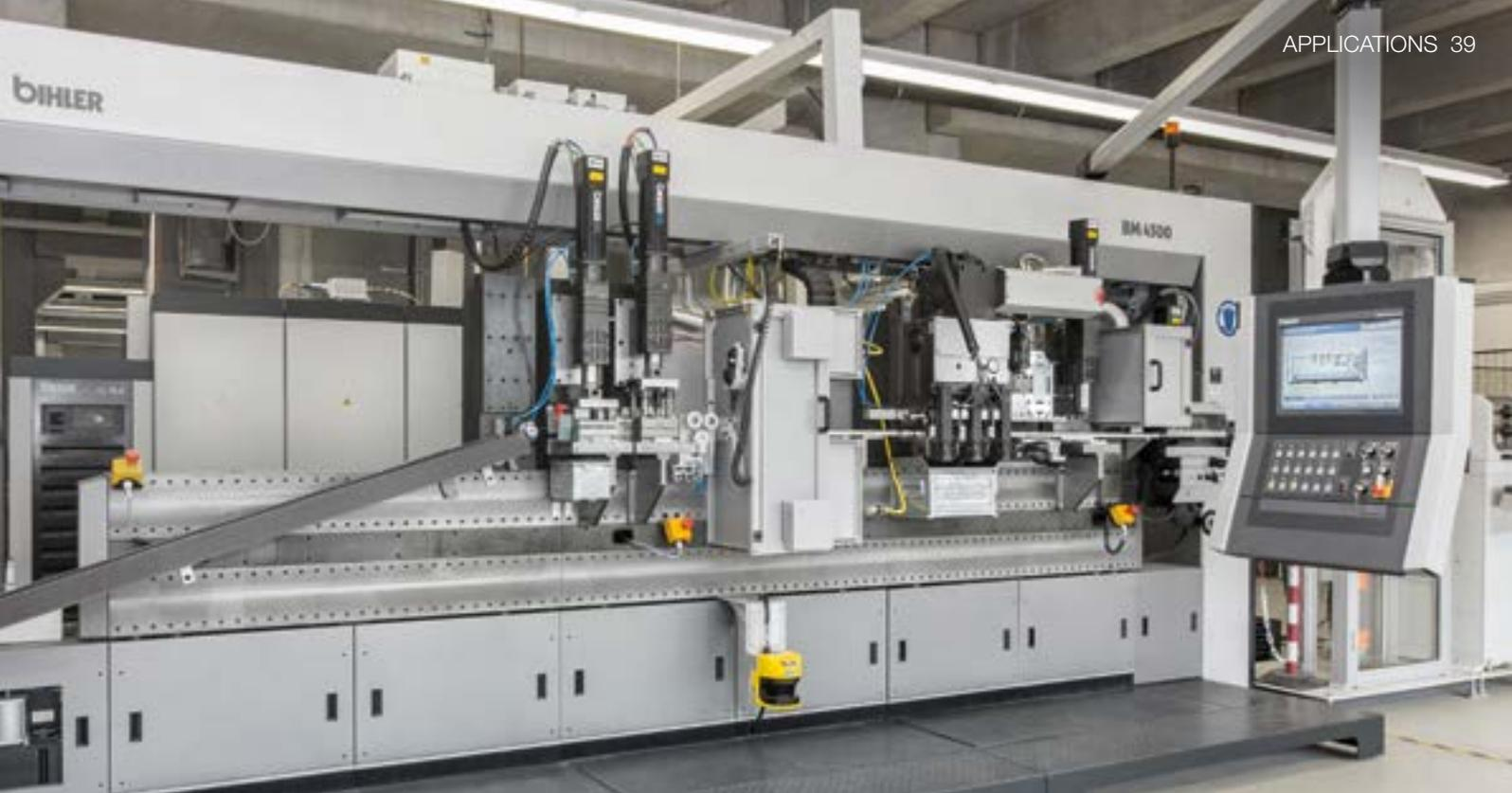
With the new BIMERIC BM 4500, it is now possible to manufacture complex stamped parts in a single, end-to-end production process. The system also features a packaging and magazinging unit.
